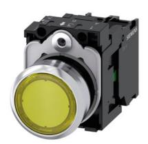
Illuminated pushbutton, 22 mm, round, metal, shiny, yellow, pushbutton, flat, momentary contact type, with holder, 1NO, LED module with integrated LED 24 V AC/DC, screw terminal, with laser labeling, upper case
