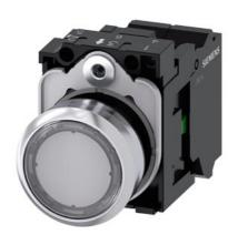
Illuminated pushbutton, 22 mm, round, metal, shiny, clear, pushbutton, flat, momentary contact type, with holder, 1NO, LED module with integrated LED 24 V AC/DC, spring-type terminal, Z=20-unit packaging
