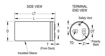
General Information Series ALS70 Dielectric Aluminum Electrolytic Description Screw Terminal, Aluminum Electrolytic RoHS AEC-Q200 No Halogen Free Yes Component 220 g Weight Dimensions D And L Include Sleeving. MS (MxH) = Notes M12x16. Mounting Clamp (Sold Separately): V4/2737 Shelf Life 156 Weeks
