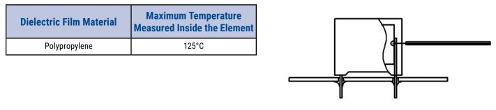
Temperature monitored inside the capacitor.
