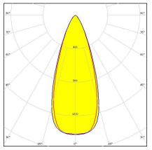
Dimensions: 26.0 mm x 26.0 mm Height: 14.74 mm ~40° wide beam 14.74 mm high lens.
