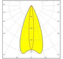
Dimensions: 26.0 mm x 26.0 mm Height: 14.96 mm ~45° x 10° oval beam. 14.96 mm high lens.
