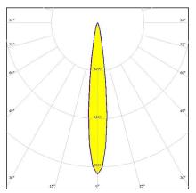
Dimensions: 26.0 mm x 26.0 mm Height: 14.74 mm ~11° diffused spot beam. 14.74 mm high lens.
