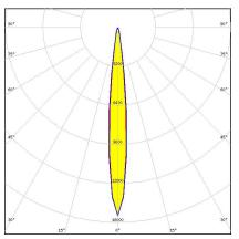
Dimensions: 26.0 mm x 26.0 mm Height: 14.82 mm ~11° smooth spot beam. 14.82 mm high lens.
