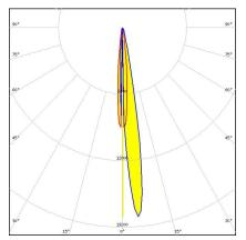
Dimensions: 26.0 mm x 26.0 mm Height: 14.83 mm ~8° beam for wall-washing. 14.83 mm high lens.
