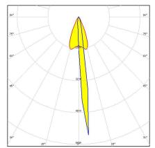
Dimensions: 26.0 mm x 26.0 mm Height: 14.95 mm ~45° x 10° oval beam for wall washing. 14.95 mm high lens.
