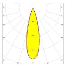
Dimensions: 26.0 mm x 26.0 mm Height: 14.88 mm ~30° medium beam. 14.88 mm high lens.
