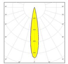
Dimensions: 26.0 mm x 26.0 mm Height: 14.85 mm ~20° medium beam. 14.85 mm high lens.
