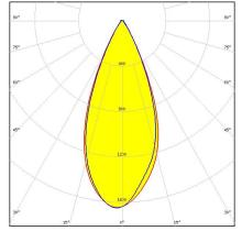
Dimensions: 26.0 mm x 26.0 mm Height: 14.74 mm ~45° wide beam. 14.74 mm high lens.
