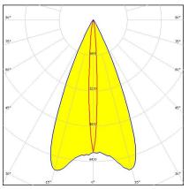
Dimensions: 26.0 mm x 26.0 mm Height: 14.97 mm ~10° x 45° oval beam. 14.97 mm high lens. Variant with beam direction rotated 90°.
