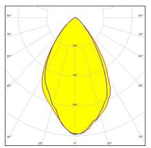
Dimensions: 26.0 mm x 26.0 mm Height: 13.43 mm ~60° wide beam. 13.43 mm high lens. Modified version to fit CREE XM-L LEDs.
