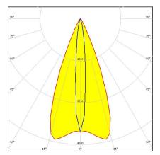
Dimensions: 26.0 mm x 26.0 mm Height: 14.97 mm ~45° x 10° oval beam. 14.97 mm high lens.
