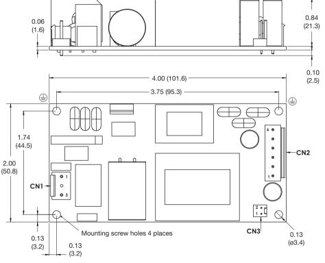
Mounting holes marked with () must be connected to safety earth for class I applications and connected together for class II applications for optimum EMC performance
