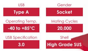
Where charging is used as the primary function for a USB connector, it's not surprising to see repeated mating and un-mating going over and above these numbers, especially for use in high traffic applications such as public charging points. **GCT** has engineered a set of full-sized USB connectors durable enough to **withstand over 20,000 cycles**, **thoroughly tested and rated**.
