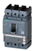
circuit breaker 3VA5 UL frame 250 3-pole, starter protection TM120M, AM, In=150A without overload protection short-circuit protection Ii=6...12 x In nut keeper kit on both sides
