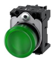
Indicator lights, 22 mm, round, plastic, green, lens, smooth, with holder, LED module, with integrated LED 24 V AC/DC, screw terminal, with laser labeling, lower case
