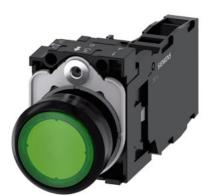
Illuminated pushbutton, 22 mm, round, plastic, green, pushbutton, flat, momentary contact type, with holder, 1 NO+1 NC, LED module with integrated LED 110 V AC, screw terminal, with laser labeling, upper case and lower case, Always upper case at the beginning of the word
