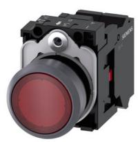
Illuminated pushbutton, 22 mm, round, plastic with metal front ring, red, pushbutton, flat, momentary contact type, with holder, 1NC, LED module with integrated LED 24 V AC/DC, spring-type terminal, Z=20-unit packaging
