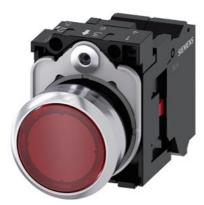
Illuminated pushbutton, 22 mm, round, metal, shiny, red, pushbutton, flat, momentary contact type, with holder, 1NC, LED module with integrated LED 230 V AC, spring-type terminal, Z=20-unit packaging
