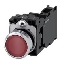
Illuminated pushbutton, 22 mm, round, metal, shiny, red, pushbutton, flat, momentary contact type, with holder, 1 NO+1 NC, LED module with integrated LED 110 V AC, spring-type terminal, with laser labeling, upper case and lower case, always upper case at beginning of line
