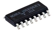
The NOMCA series features a standard 14 pin or 16 pin narrow body (0.150") small outline SMT package. The network is constructed with tantalum nitride resistor film on high purity alumina substrate for improved ESD and moisture protection. Custom schematics are available consult factory.
