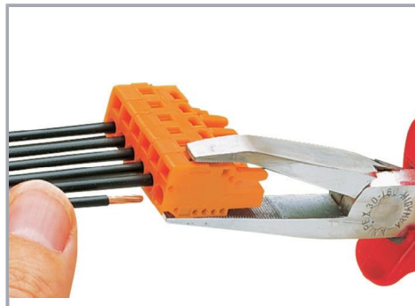
Inserting a conductor via operating tool.
