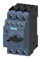
Circuit breaker size S0 for motor protection, CLASS 10 A-release 9...12.5 A N-release 163 A screw terminal Standard switching capacity with transverse auxiliary switches 1 NO+1 NC
