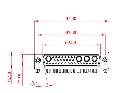
THIS IS A C.A.D. GENERATED DRAWING TOLERANCE UNLESS OTHERWISE SPECIFIED DO NOT MAKE MANUAL REVISIONS TO MASTER. .X ±0.25 .XX ±0.13
