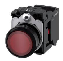
Illuminated pushbutton, 22 mm, round, plastic, red, pushbutton, flat, momentary contact type, with holder, 1NC, LED module with integrated LED 230 V AC, spring-type terminal, with laser labeling, upper case
