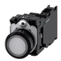
Illuminated pushbutton, 22 mm, round, plastic, clear, pushbutton, flat, momentary contact type, with holder, 1 NO+1 NC, LED module with integrated LED 24 V AC/DC, spring-type terminal, with laser labeling, inscription or symbol Customer-specific selection with SIRIUS ACT configurator (CIN)
