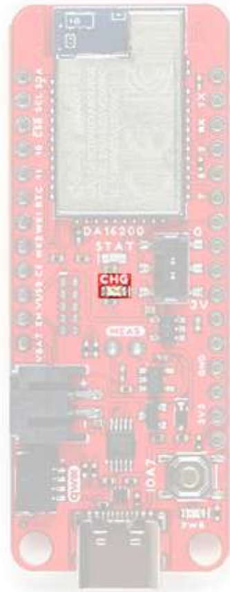
The battery charging ( CHG ) LED indicator on the DA16200 Thing Plus. (Click to enlarge)
