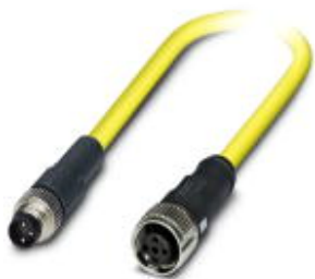
Sensor/actuator cable, 3-position, PVC, yellow, Plug straight M8, on Socket straight M12 SPEEDCON, A-coded, cable length: 0.5 m
