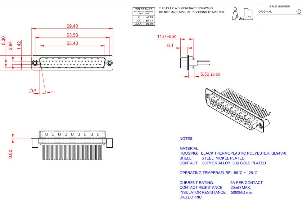
WITHSTANDING VOLTAGE: 1000V AC rms
