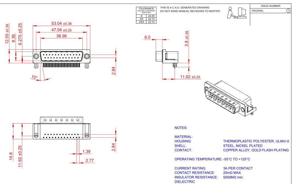
WITHSTANDING VOLTAGE: 1000V AC rms
