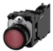
Illuminated pushbutton, 22 mm, round, plastic, red, pushbutton, flat, momentary contact type, with holder, 1 NO+1 NC, LED module with integrated LED 110 V AC, spring-type terminal, with laser labeling, symbol number according to, ISO 7000 or IEC 60417
