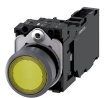
Illuminated pushbutton, 22 mm, round, plastic with metal front ring, yellow, pushbutton, flat, momentary contact type, with holder, 1 NO+1 NC, LED module with integrated LED 230 V AC, screw terminal, with laser labeling, upper case and lower case, always upper case at beginning of line
