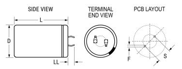
**General Information** Series ALC40 Dielectric Aluminum Electrolytic Description Snap-In, Aluminum Electrolytic RoHS Lead 2 Pin AEC-Q200 No Component Weight 131 g Shelf Life 156 Weeks
