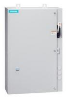
Non-reversing motor starter Size 3 Three phase full voltage Solid-state overload relay OLRelay amp range 25-100A 24Vdc coil Combination type 100A non-fusible disconnect Encl NEMA type 4X 316 S-steel Water/dust tight non-corrosive Standard width enclosure
