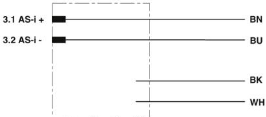
Contact assignment of the AS-Interface distributor
