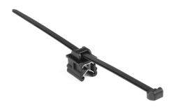
Outside Serrated Cable Tie & Edge Clip, 6.0" Long, EC9, 1-3 mm Panel, 50lb, PA66HS, Black, 500/pkg
