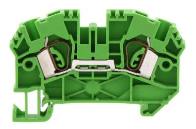
Feed-through terminal, Tension-spring connection, Mounting type: Mounting rail TS 35/7.5, Rated cross-section: 4 mm², Width: 6.1 mm, Colour: Green
