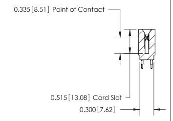
ACAD REFERENCE NO. 745 Series Ultra-Mate Card Edge Connector - Press Fit DRAWN: J.LEE Part Number: 745-072-525-201 CHECKED: **EDAC INC** SCALE: THESE DRAWINGS AND SPECIFICATIONS ARE THE PROPERTY OF EDAC INC.,AND TORONTO, ONTARIO SHALL NOT BE REPRODUCED, OR COPIED DRAWING NUMBER CANADA OR USED AS THE BASIS FOR THE 745-ENG MASTER MANUFACTURE OR SALE OF APPARATUS YOUR CONNECTION TO QUALITY & SERVICE WITHOUT WRITTEN PERMISSION.
