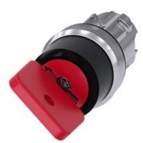
Key-operated switch O.M.R, 22 mm, round, metal, shiny, lock number 73037, red, with 2 keys, 2 switch positions O-I, latching, actuating angle 90°, 10:30h/13:30h, key removal O, with laser labeling, upper case
