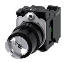
RONIS key-operated switch, 22 mm, round, plastic, Lock No. SB30, with 2 keys, 2 switch positions O-I, latching, 10:30/1:30 o'clock, key removal O+I, with holder, 1NO, spring-type terminals, possible special locks: SB31, 421, 455, Z=20-unit packaging
