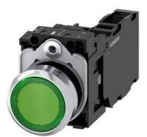
Illuminated pushbutton, 22 mm, round, Metal, shiny, green, pushbutton, flat, momentary contact type, with holder, 1 NO+1 NC, LED module with integrated LED 230 V AC, screw terminal, with laser labeling, symbol number according to, ISO 7000 or IEC 60417
