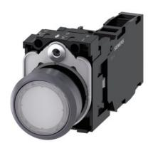
Illuminated pushbutton, 22 mm, round, plastic with metal front ring, white, pushbutton, flat, momentary contact type, with holder, 1 NO+1 NC, LED module with integrated LED 110 V AC, screw terminal, with laser labeling, upper case
