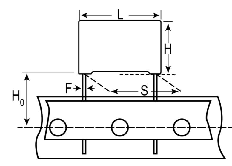
Click <u>here</u> for the 3D model. **Dimensions** L 13mm +0.2/-0.5mm H 9mm +0.1/-0.5mm
