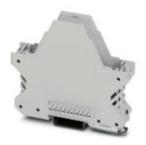
DIN rail housing, Lower housing part with metal foot catch, flat design, with vents, width: 22.6 mm, cross connection: integrated bus connector, number of positions cross connector: 10, color: light gray (7035)
