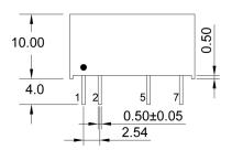
Note: Unit: mm[inch] Unless otherwise specified, all tolerances: ± 0.25mm
