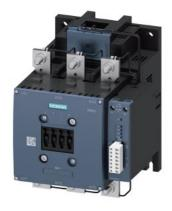
Contactor, AC-1, 400 A/690 V/40  $^{\circ}$ C, S10, 3-pole, 96-127 V AC/DC, PLC-IN optional, with varistor, 1 NO+1 NC, connection bar/ screw terminal, remaining life time
