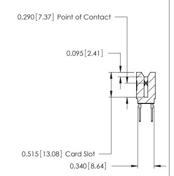
ACAD REFERENCE NO. 746 Series Ultra-Mate Card Edge Connector - Press Fit DRAWN: J.LEE Part Number: 746-016-527-206 CHECKED: **EDAC INC** SCALE: THESE DRAWINGS AND SPECIFICATIONS ARE THE PROPERTY OF EDAC INC.,AND TORONTO, ONTARIO SHALL NOT BE REPRODUCED, OR COPIED DRAWING NUMBER CANADA OR USED AS THE BASIS FOR THE 746-ENG MASTER MANUFACTURE OR SALE OF APPARATUS YOUR CONNECTION TO QUALITY & SERVICE WITHOUT WRITTEN PERMISSION.
