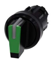
Selector switch, illuminable, 22 mm, round, plastic, green, selector switch, short, 3 switch positions I-O-II, latching, actuating angle  $2x45^{\circ}$ , 10:30h/12h/13:30h, with laser labeling, upper case
