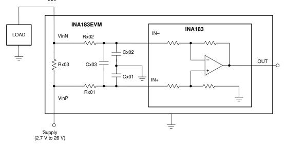
Figure 3-1. Measurement With Shunt
