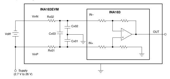
Figure 3-2. Measurement Without Shunt
