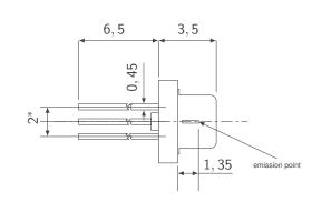
all dimensions in mm. Tolerance  $\pm 0,\, 1$  except given ones \* at the bottom of the LED
