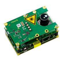
Thanks to a simple supply system, with only 3 positive voltage domains, the sensor simplifies the design of the supply unit and together with a low power dissipation allows a very compact 3D camera.
