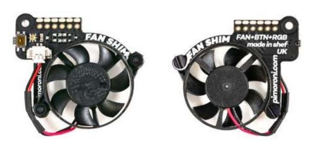
Make your Raspberry Pi 4 *seriously* cool with Fan SHIM! This 30mm no-solder, controllable CPU fan with RGB LED and tactile switch will give your Raspberry Pi significantly better thermal performance. It's whisper-quiet too!
