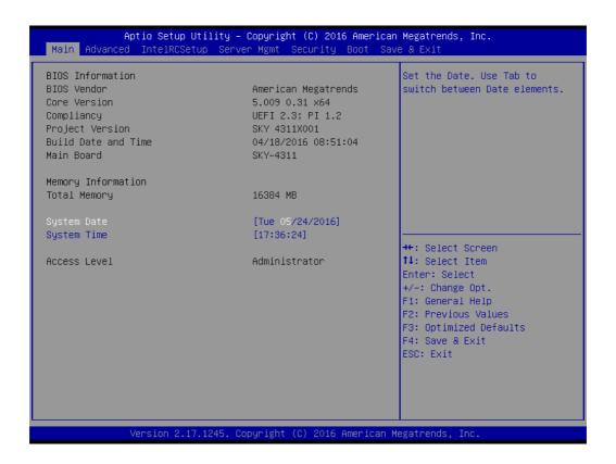
The Main BIOS setup screen has two main frames. The left frame displays all the options that can be configured. Grayed-out options cannot be configured; options in blue can be. The right frame displays the key legend. Above the key legend is an area reserved for a text message. When an option is selected in the left frame, it is highlighted in white. Often a text message will accompany it.
