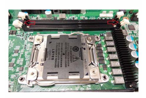
3. Align the memory module with the slot. When inserted properly, the memory slot locking levers lock automatically into the indentations at the ends of the module. Follow the recommended memory population table (page 9) to install additional memory modules.
