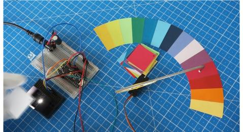
Identifying specific colors with a color sensor is not as simple as pointing the sensor at a color patch and taking a reading. There are many factors such as distance, field of view and ambient lighting conditions that can affect readings. Adafruit forum member systembolaget has developed a system capable of quickly and reliably identifying many different colors and has put together an excellent tutorial on the subject.
