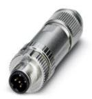
Bus system connector, PROFIBUS (12 Mbps), 2-position, shielded, Plug straight M12 SPEEDCON, B-coded, Spring-cage connection, knurl material: Zinc die-cast, nickel-plated, external cable diameter 4 mm ... 8 mm
