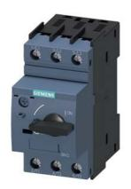
special type circuit breaker size S00 for transformer protection A-release 5.5...8 A short-circuit release 163 A screw terminal standard switching capacity ambient temperature -50 °C 500 switching cycles
