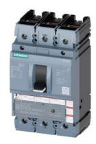
circuit breaker 3VA5 UL frame 250 breaking capacity class M 35kA @ 480 V 3-pole, line protection TM230, FTAM, In=125A overload protection Ir=125A fixed short-circuit protection Ii=5...10 x In cable connection on both sides
